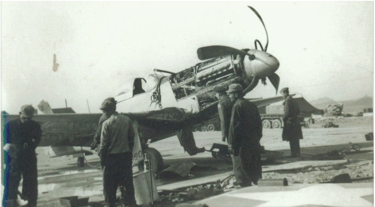
Mustang 350 after the undercarriage collapsed upon landing.
