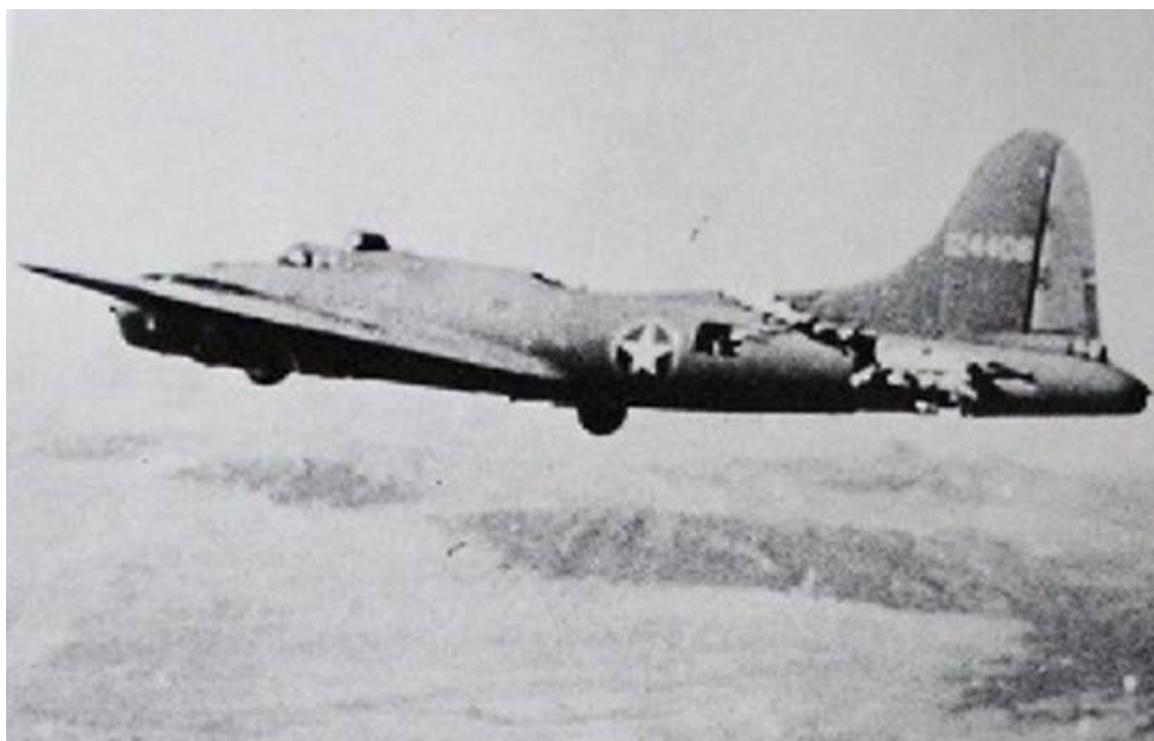
Although the tail actually bounced and swayed in the wind and twisted when the plane turned and all the control cables were severed, except one single elevator cable still worked, and the aircraft still flew – miraculously! The tail gunner was trapped because there was no floor connecting the tail to the rest
